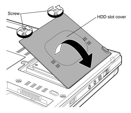
Figure 4-6 Removing the HDD slot cover
